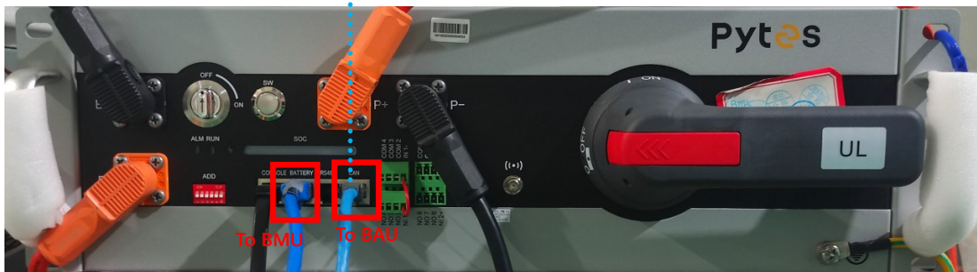
Pic 1.1.4 CAN port on BCU
